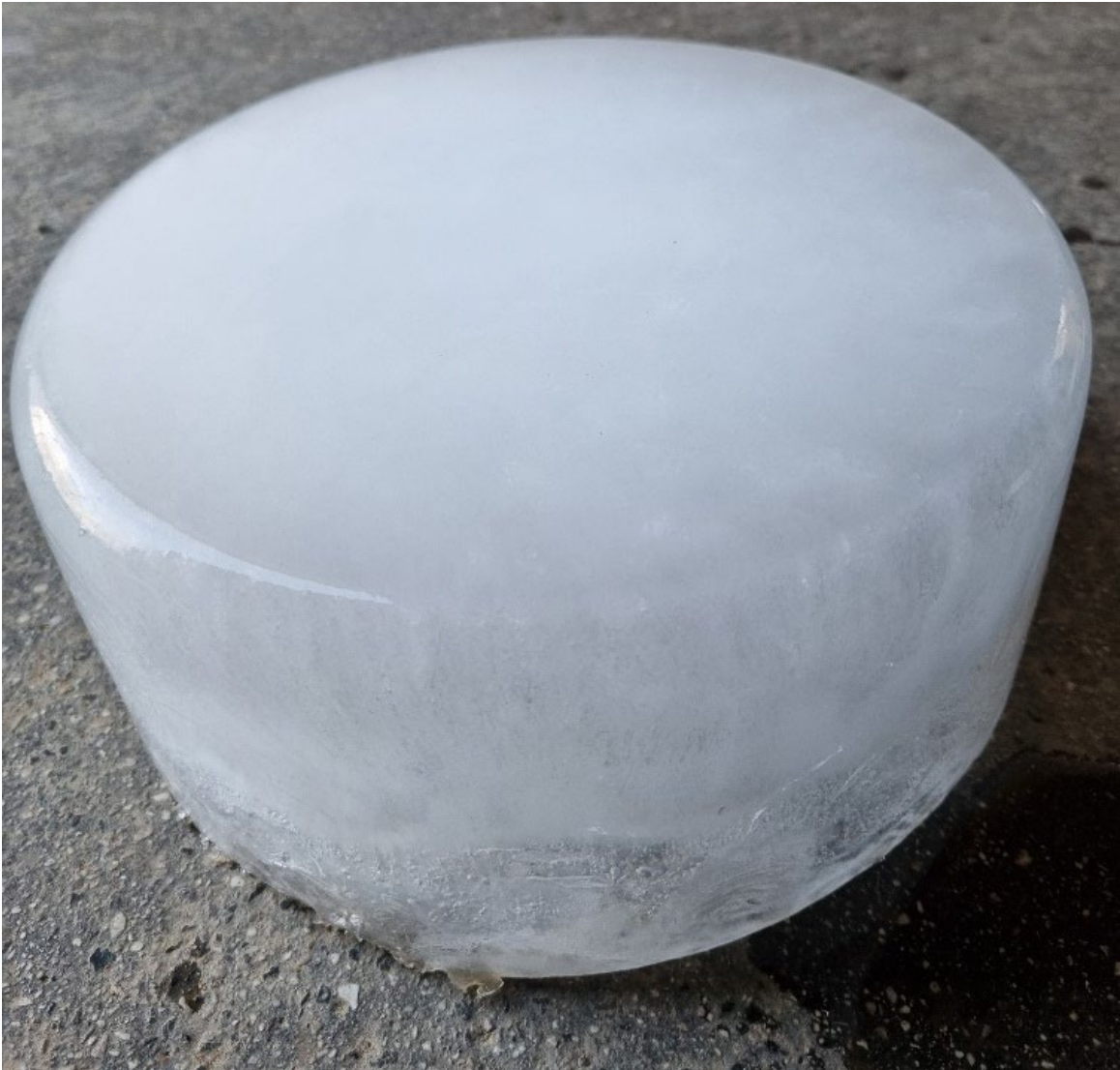
Figure 3: artificial ice block used for testing with a diameter of 25 cm
